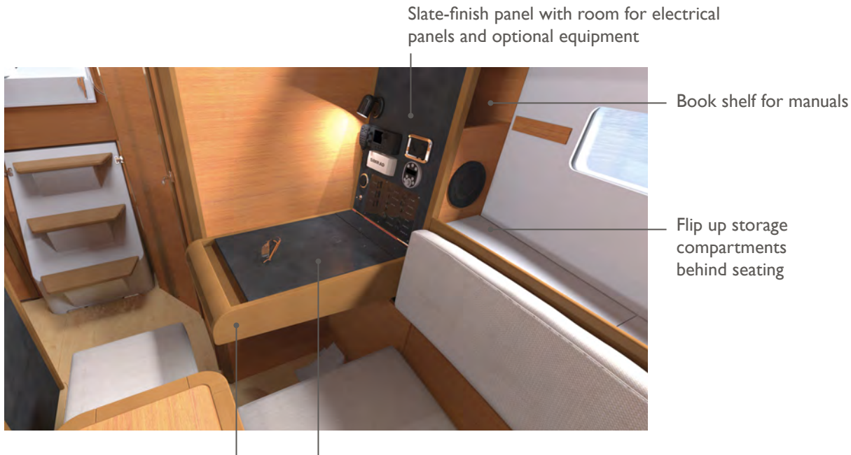
Nav station hinges up and out of the way when dining or to create a longer berth to port
