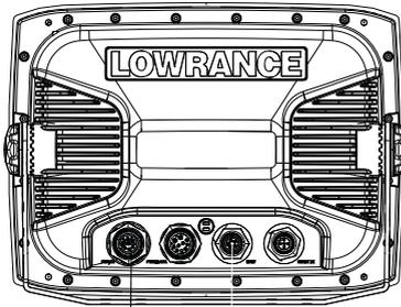
Connect Yellow wire to the yellow accessory wake up wire of the HDS. SonicHub will turn on when the HDS is turned on.
