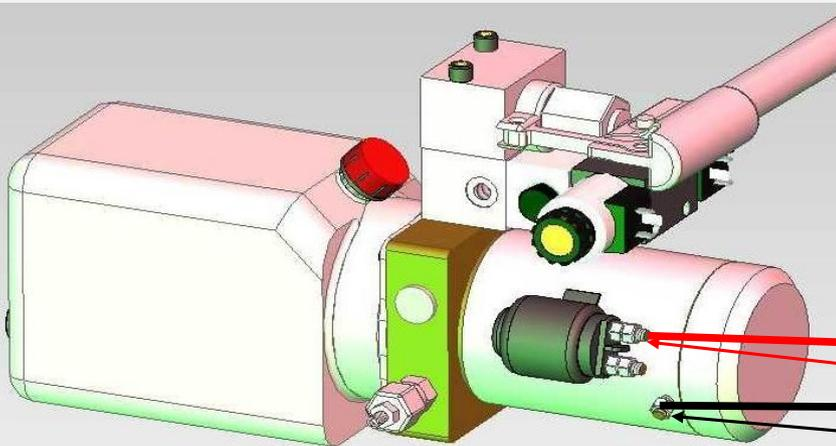
Check that power pack is supply ( U=12V) by using a Voltmeter between Input Relay terminal ( red Cable ) and 0V Motor Terminal ( Black cable )
